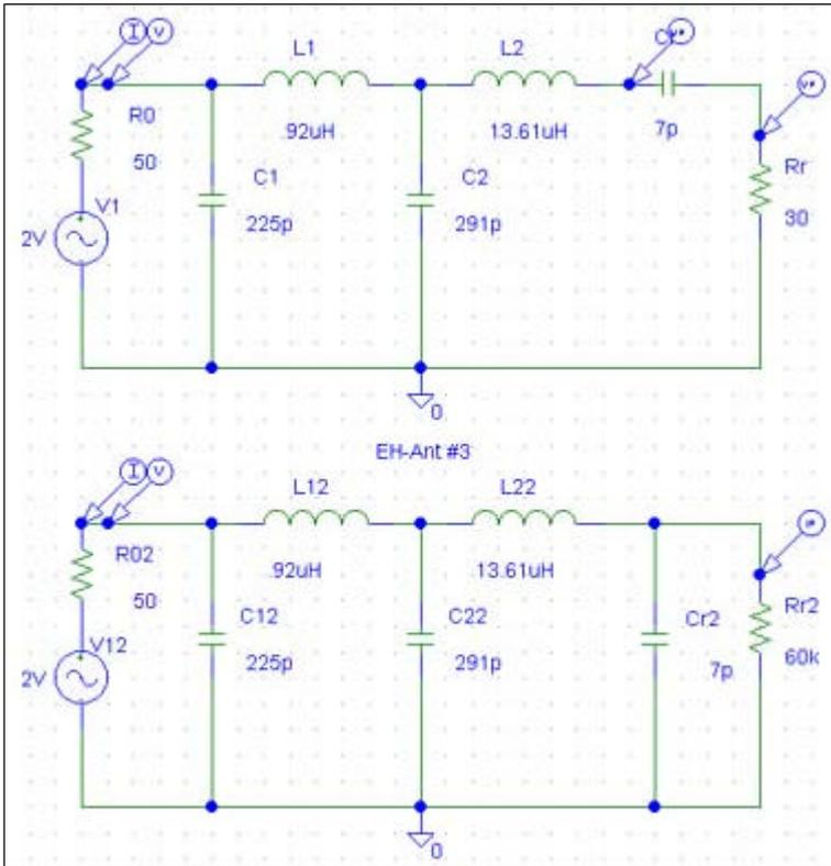
The two circuits are exactly the same, and they produce the same plot. Change only the way to see the circuit from computing method.
