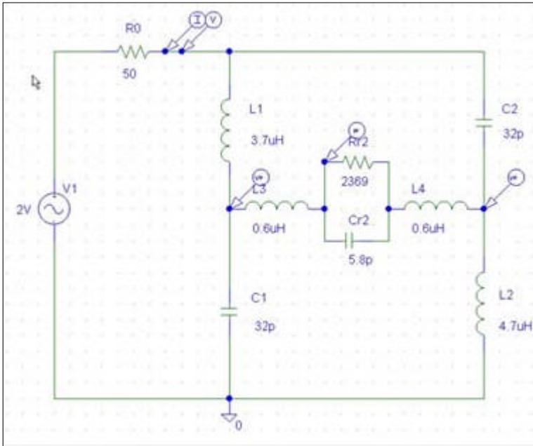
This is the diagram equivalent of #2 EH-Antenna.
